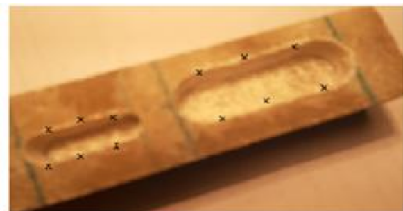
Fig. (1) Defects at groove walls surfaces.
