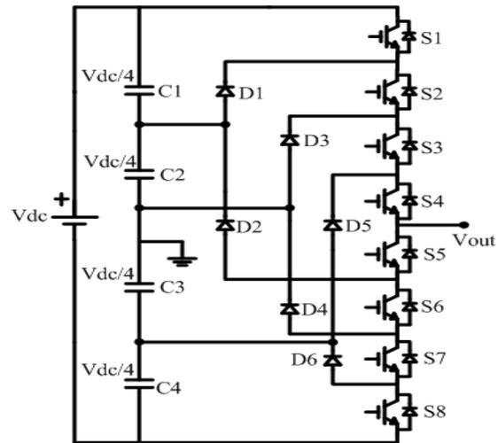
Fig. 1 Five-level NPC inverter
