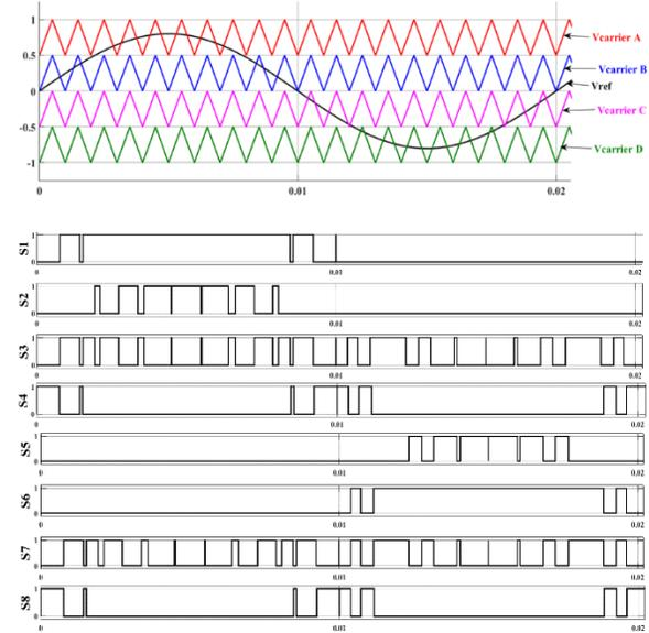
Fig. 6 PWM switching pattern of proposed topology
