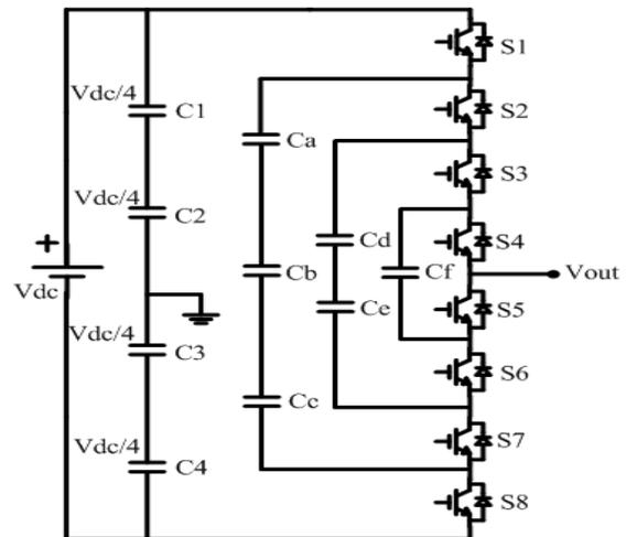
Fig. 2 Five-level FC inverter
