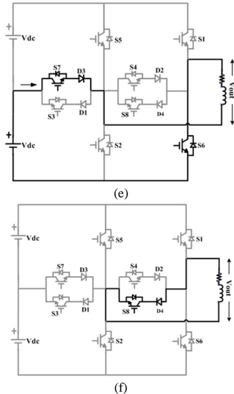
Fig. 5 Modes of operation a) Mode 1,  $V_{out}=+2V_{dc}$  b) Mode 2,  $V_{out}=+V_{dc}$  c) Mode 3,  $V_{out}=0$  d) Mode 4,  $V_{out}=-2V_{dc}$  e) Mode 5,  $V_{out}=-V_{dc}$  f) Mode 6,  $V_{out}=0$
