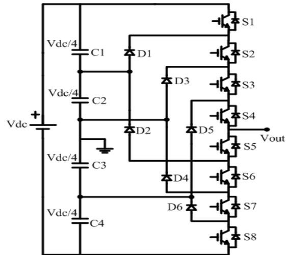
Fig. 1 Five-level NPC inverter
