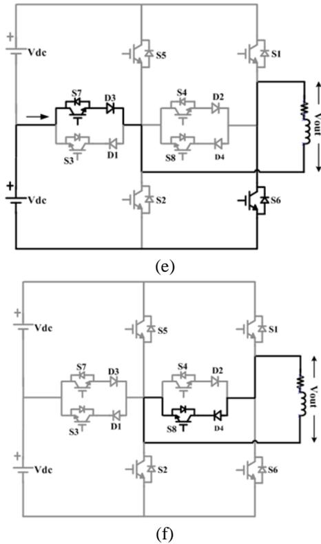
Fig. 5 Modes of operation a) Mode 1,  $V_{out}=+2V_{dc}$  b) Mode 2,  $V_{out}=+V_{dc}$  c) Mode 3,  $V_{out}=0$  d) Mode 4,  $V_{out}=-2V_{dc}$  e) Mode 5,  $V_{out}=-V_{dc}$  f) Mode 6,  $V_{out}=0$
