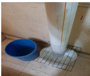
Figure (4) Permeability Test (Simple Falling Head Apparatus) [1]
