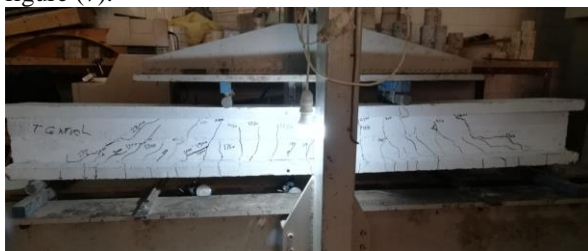
Figure 7: Beam under loading.
