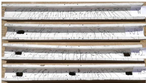
(a) Beams of the group (A) with welded mesh.
