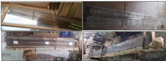
(A) Beams reinforced with welded metal mesh.
