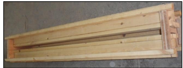
Figure 4: The shape of the I-beam mold.
