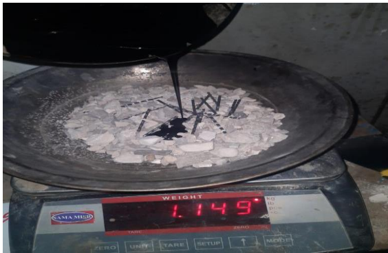
Figure (3): Modified HMA Preparation
