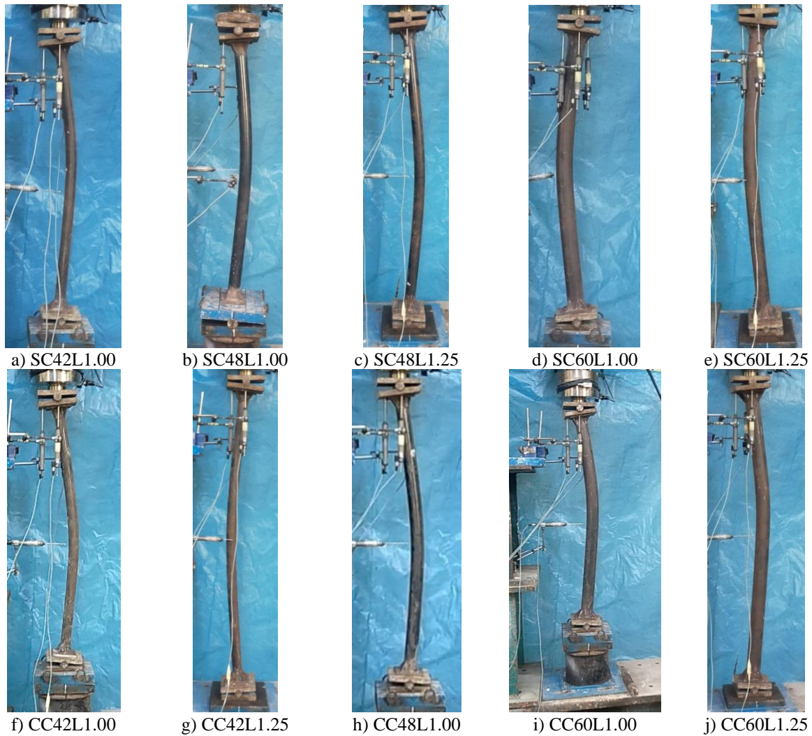
Figure 7 – Experimental failure mode shape for slender column specimens.
