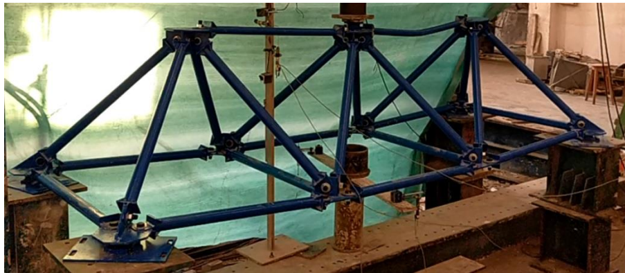
Figure 10 – Failure Mode Shape of Steel Space Truss ST2.
