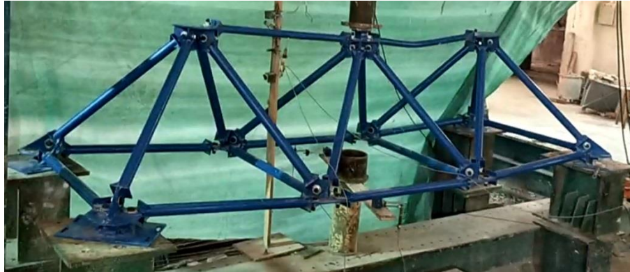
Figure 12– Failure Mode Shape of Steel Space Truss CT2.
