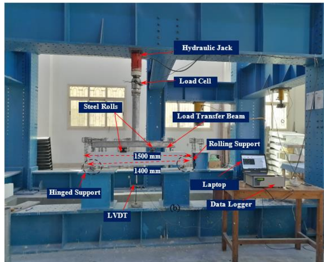
Figure4- Four-point loading test set-up.
