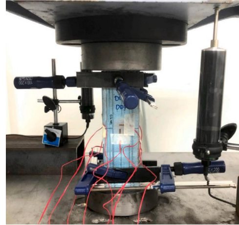
Figure 4- a. Built-up cross-sections configurations, b. The Test set-up by Teoh et al [34]
