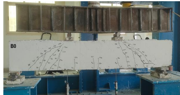
Fig. 7. Failure Mode of The Control Beam B0
