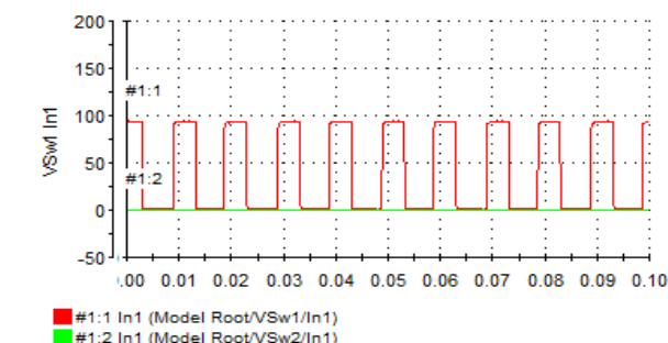
i. Voltage stress of S_1 at f_{sw} = 100\text{Hz}
