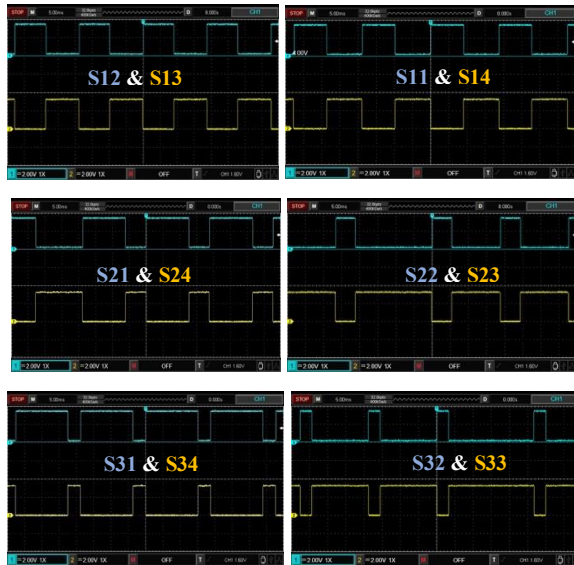
Figure 10- Raspberry Pi Pico DSP board control signals as the output pulses on the switches' gates.
