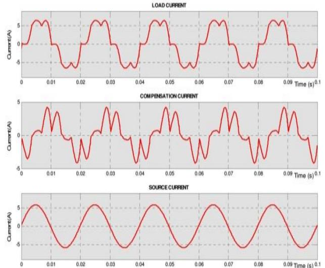
Fig. 10 Current waveform under ideal condition
