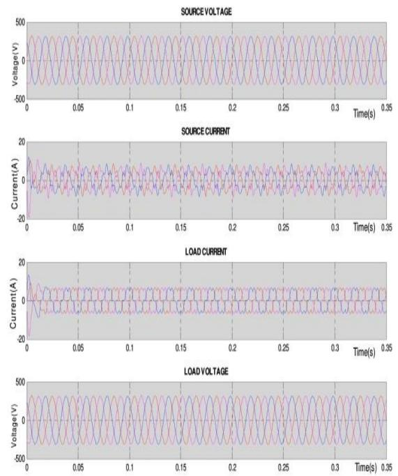
Fig. 6 Voltage and current waveform with 5th-tune passive filter
