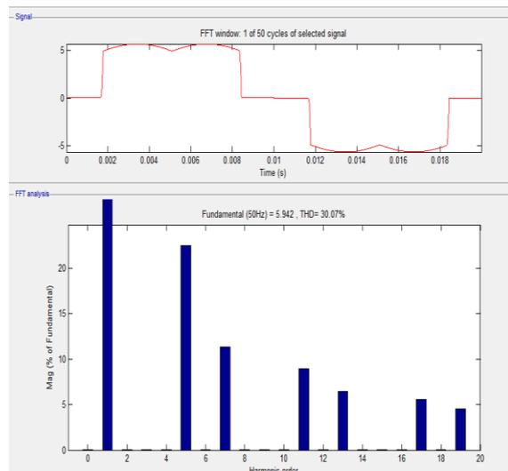
Fig.10 FFT-analysis of load current without APF
