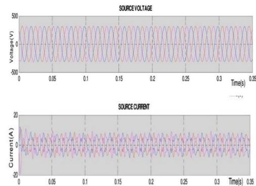
Fig.7 Voltage and current waveform with 7th-tune passive filter
