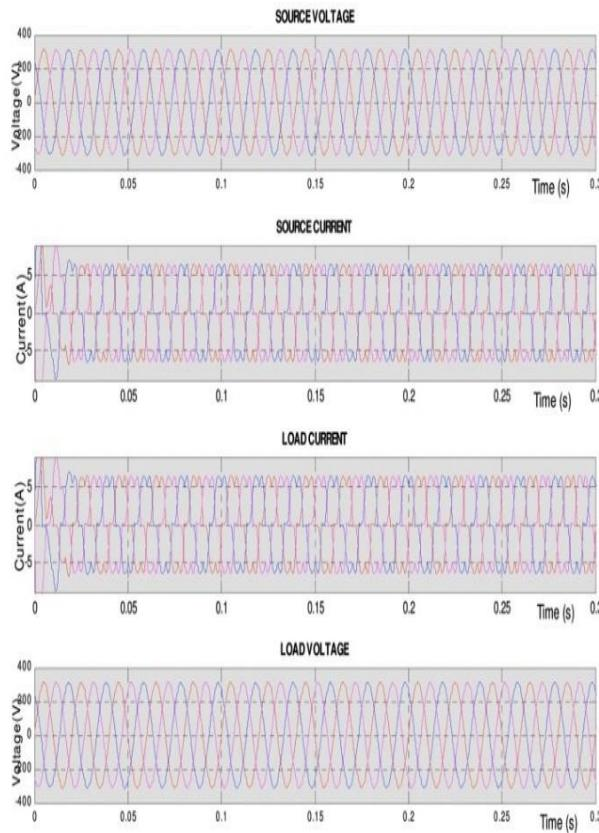
Fig.5 Voltage and current waveform without Compensation
