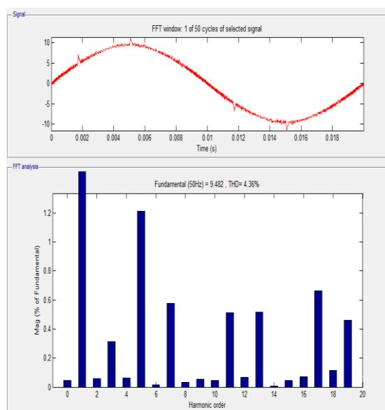
Fig.11 FFT analysis of load current with APF
