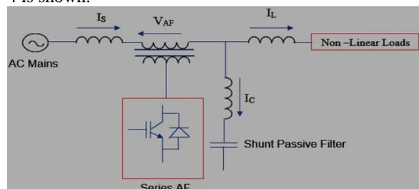
Fig.1 hybrid filter type
