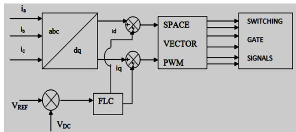
Fig .2 Control block diagram of Fuzzy based SVPWM
