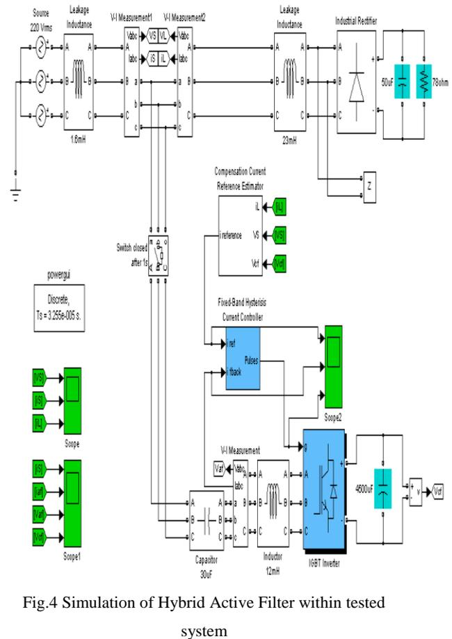
Fig.4 Simulation of Hybrid Active Filter within tested system
