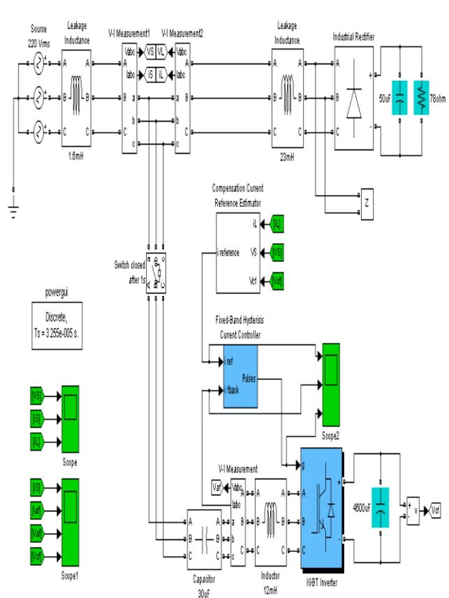
Fig.4 Simulation of Hybrid Active Filter within tested system
