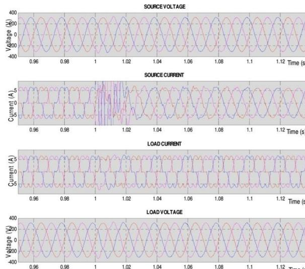
Fig.8 Voltage and current waveform with hybrid active filter
