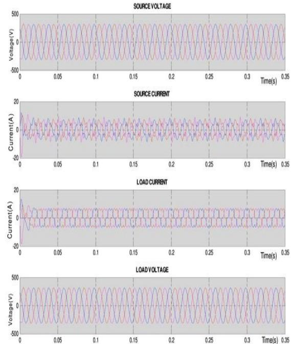
Fig. 6 Voltage and current waveform with 5th-tune passive filter
