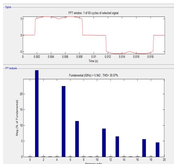
Fig.10 FFT-analysis of load current without APF
