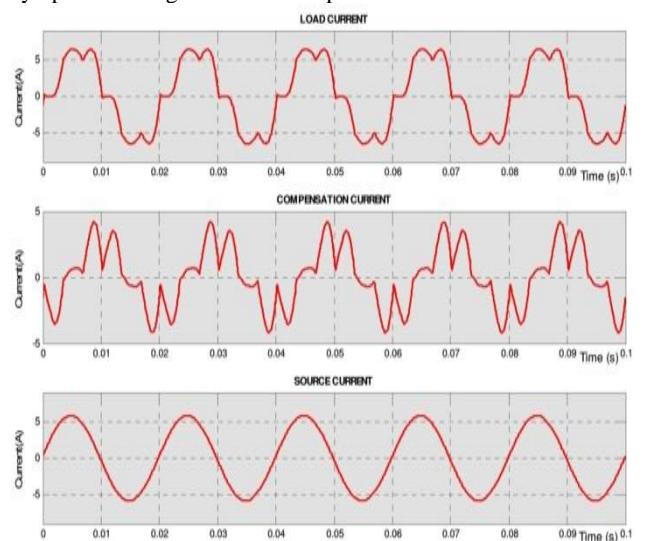
Fig. 10 Current waveform under ideal condition
