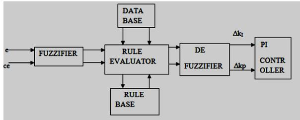
Fig .3 Block diagram of Fuzzy Logic Controller
