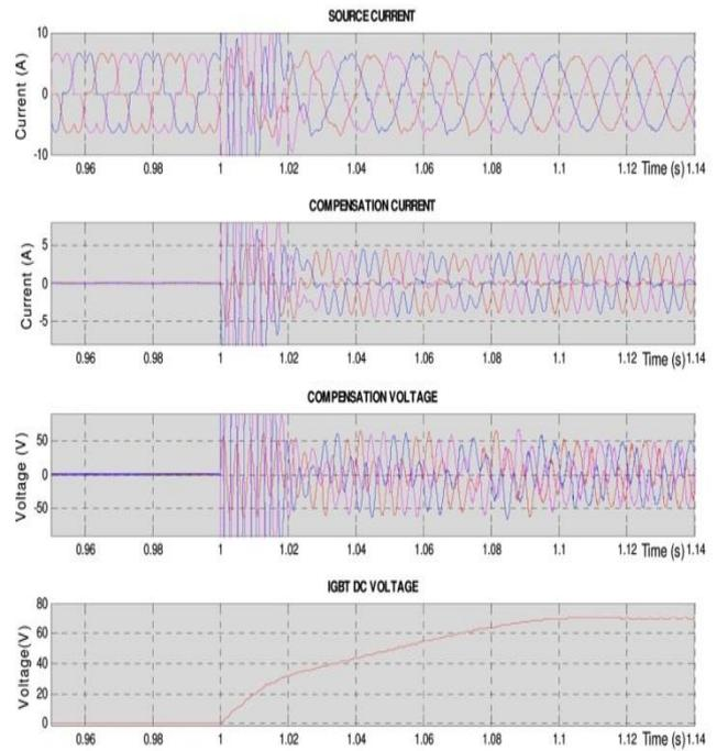
Fig. 9 Voltage and current waveform at IGBT Inverter power line
