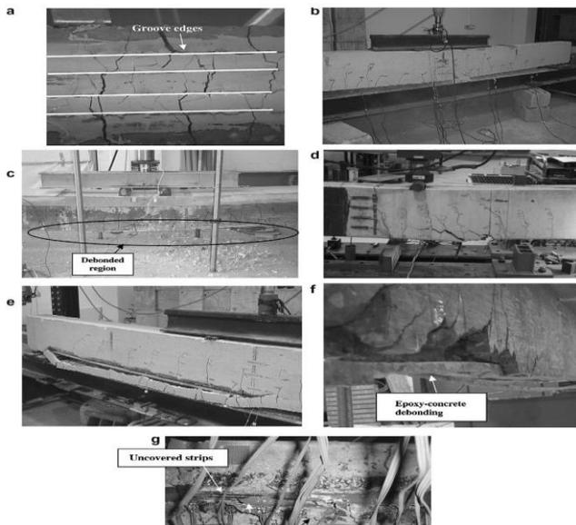
Fig. 11: Debonding failure modes of strengthened RC beams using NSM techniques [24].
