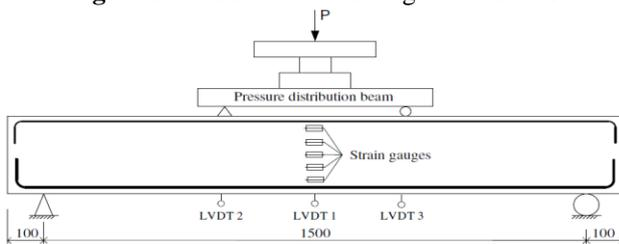
Fig. 6: Locations of equipment along the tested beams.
