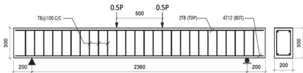
Fig. 12 : Test setup of tested beams [25].
