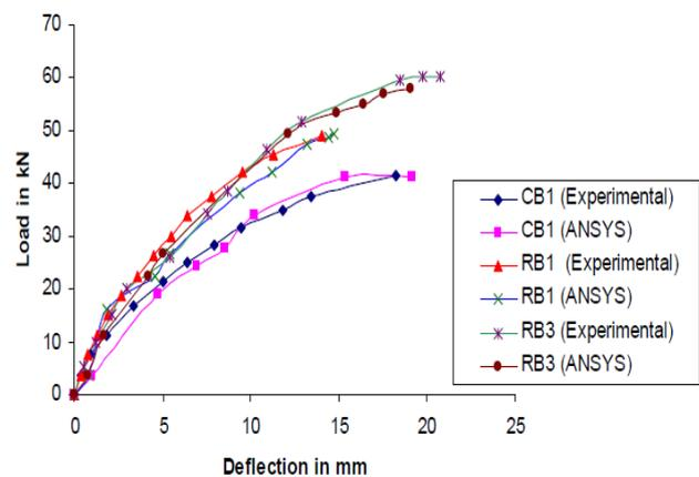
Fig. 4: Experimental and FEM load-deflection curves for beams [18].
