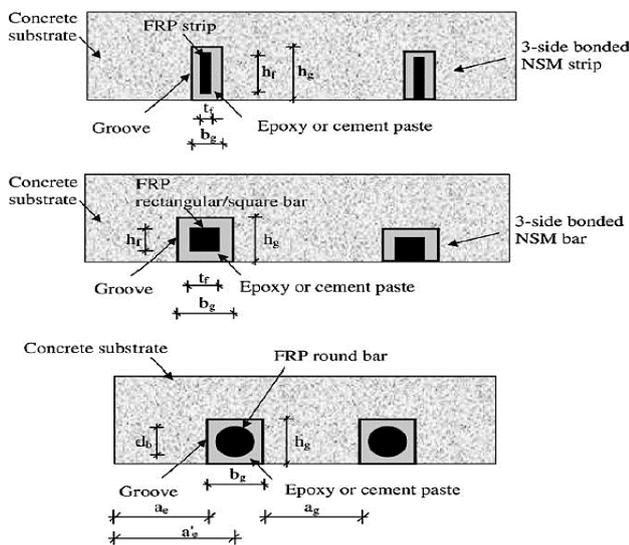
Fig. 8: Different NSM FRP installation and grooving details [13].
