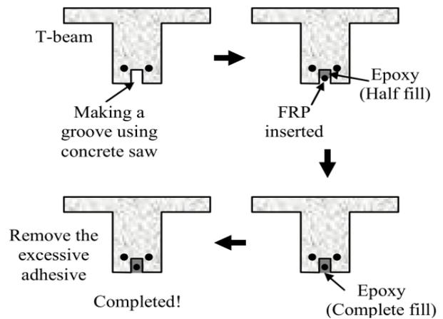
Fig. 9: Detailed procedures of NSM strengthening technique [17].
