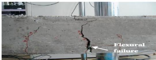
A) Flexural failure of the control specimen.
