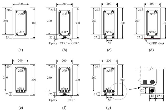
Fig. 13: tested beams cross sectional details [25].
