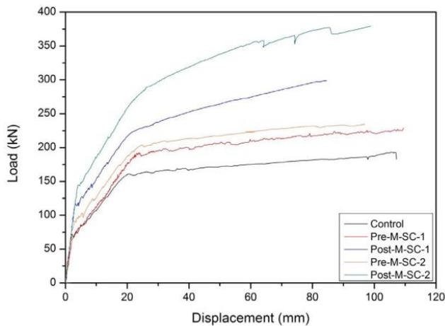
Fig. 21: Load-Deflection behaviour of the tested beams [37].
