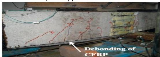
C) CFRP debonding from mid-Span.
