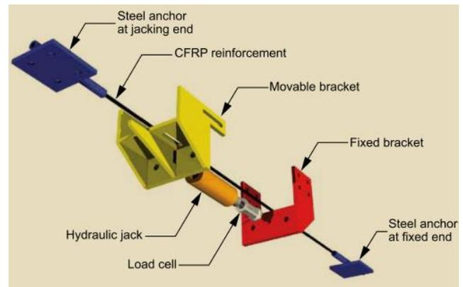
Fig. 19: Components of prestressing system [34].
