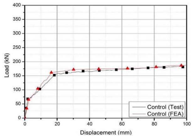
Fig. 23: Comparison of Experimental and FEA load – deflection curve for control beam [37].
