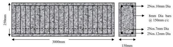
**Fig. 17:** Details of reinforcement of beams specimens [33].
