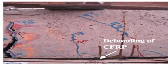
D) CFRP debonding under the loading point.
