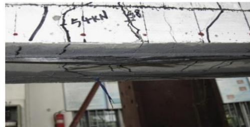
C) Rupture of CFRP strips.
