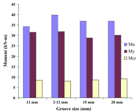
**Fig. 14:** Effect of groove size on the ultimate moment capacity [30].
