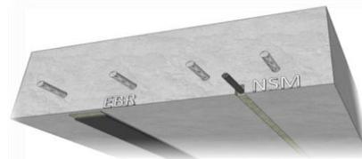
Fig. 1: (EB) and (NSM) Flexural strengthening technique.
