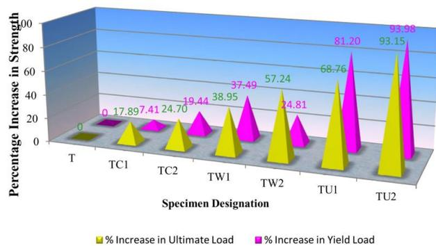
Fig. 18: Effect of GFRP plating on strength for t-series beams [33].
