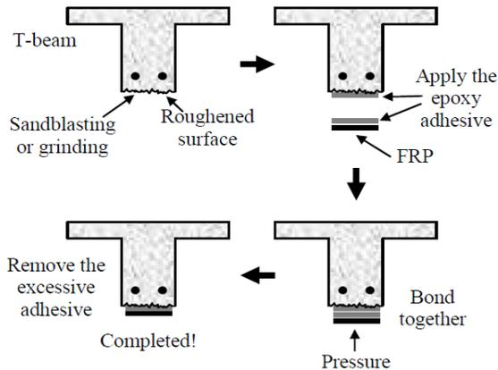
Fig. 2: Detailed procedures of EB strengthening technique [17].
