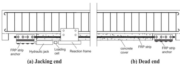
**Fig. 15:** Strengthening and pre-stressing system of the tested beam [32].
