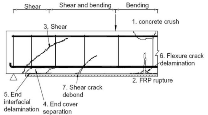
Fig. 3: Failure modes of EB strengthened beams [17].
