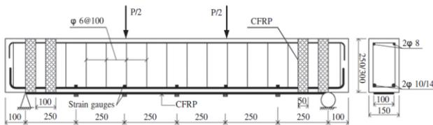
Fig. 5: Details of flexural strengthened beams.
