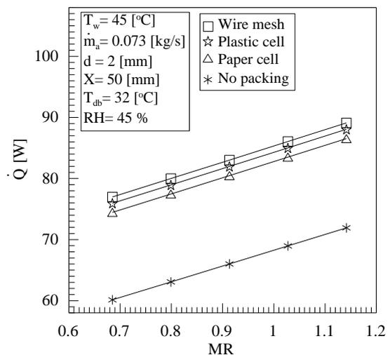
Fig. (16). Rejected heat versus water/air mass flow ratio (MR) with and without packing
