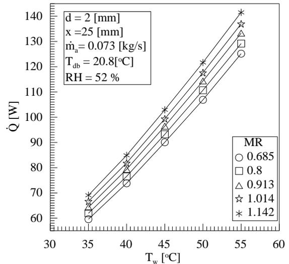
Fig. (3). Effect of water inlet temperature on the rejected heat for different mass flow rate ratio.
