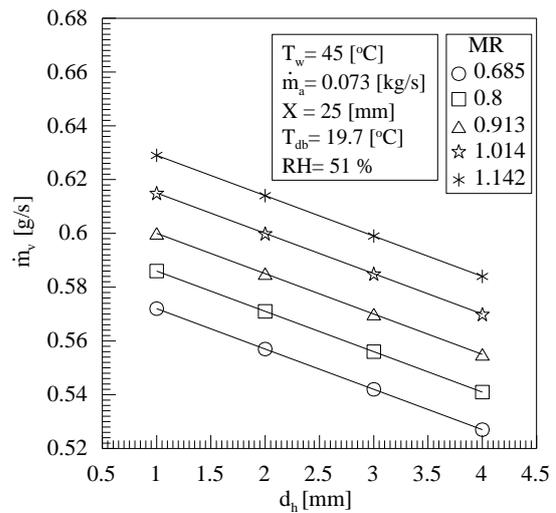
Fig. (11). Effect of injection holes diameter on the vaporization rate for different mass flow rate ratio.
