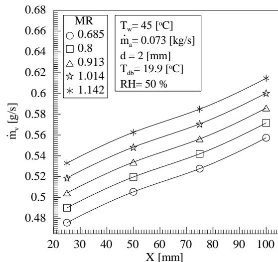
Fig. (14). Effect of interval distance between injection holes on the vaporization rate for different mass flow rate ratio
