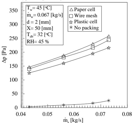
Fig. (18). Effect air mass flow rate on the pressure drop ( $\Delta P$ ) at different types of packing.
