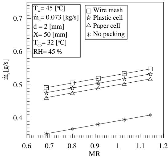
Fig. (17). Vaporization rate versus water/air mass flow ratio (MR) with and without packing.
