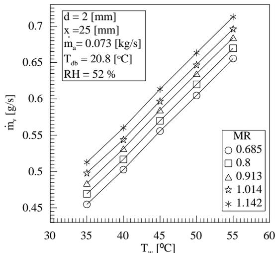
Fig. (5). Effect of water inlet temperature on the vaporization rate for different mass flow rate ratio.
