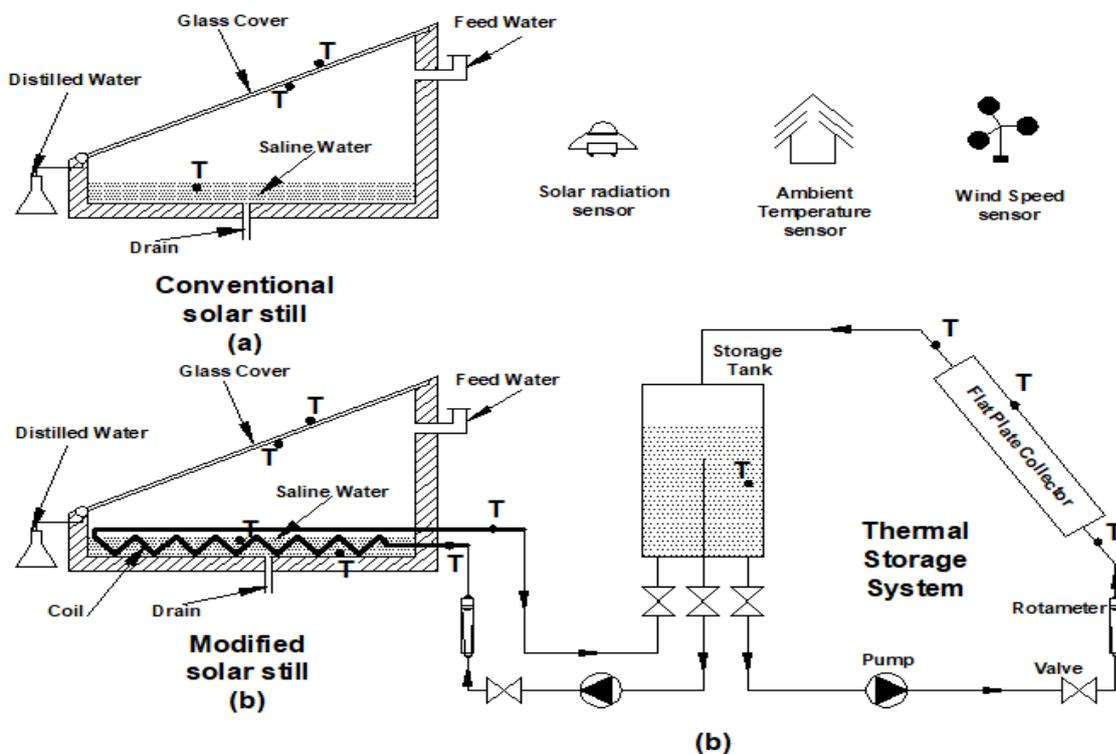
**Fig. 1. Layout of the experimental set-up.**
