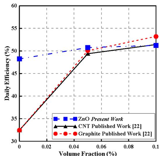
Fig. 19 Present experimental data of daily efficiency and data of Otanicar [22]
