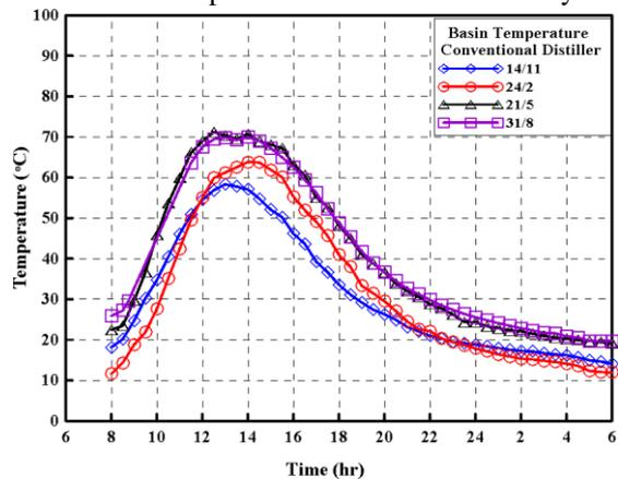
Fig. 9 Basin temperatures of conventional distiller
