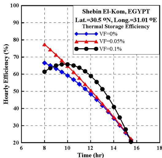
Fig. 17. Variation of hourly efficiency of thermal storage system for different volume fractions of nanoparticles
