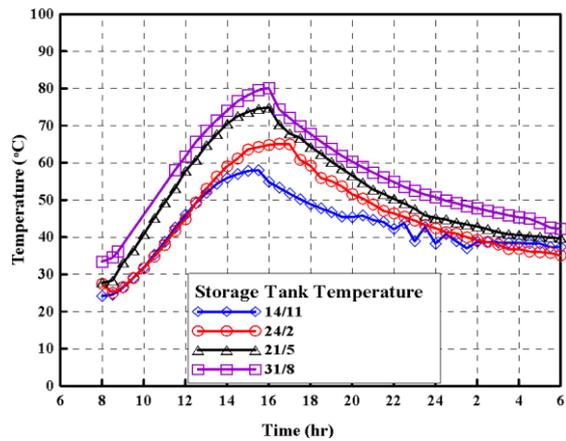
Fig. 8 Thermal storage tank temperatures
