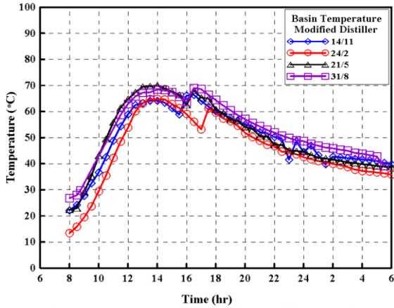
Fig. 10 Basin temperatures of modified distiller
