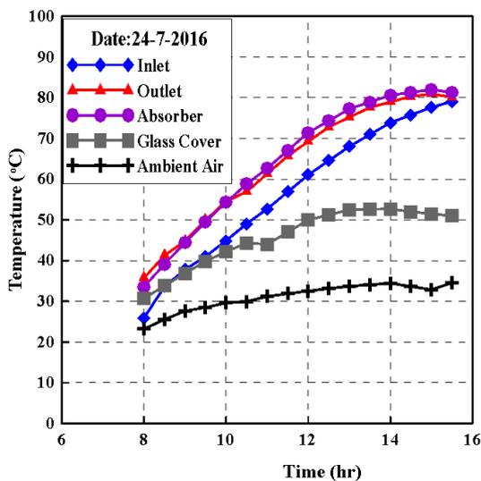
Fig. 7 Measured temperatures of flat plate solar collector
