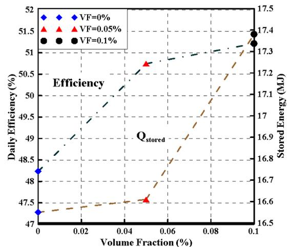
Fig. 18. Effect of nanoparticles volume fraction on the daily efficiency and stored heat in the storage tank.
