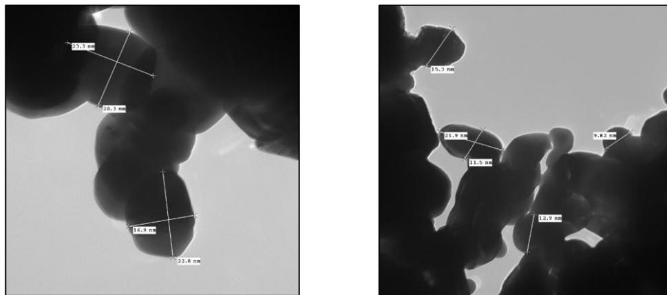
**Fig. 5. TEM images of prepared ZnO nanoparticles.**
