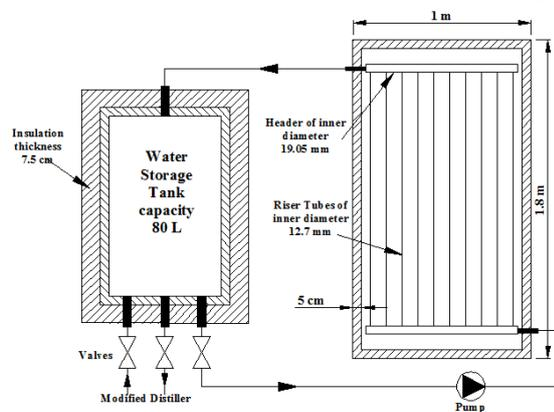
Fig. 3. Schematic diagram of the thermal storage system
