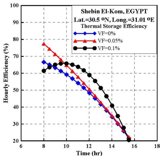
Fig. 17. Variation of hourly efficiency of thermal storage system for different volume fractions of nanoparticles
