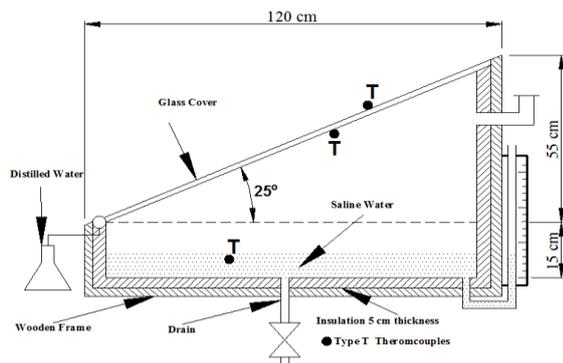
Fig. 2. Schematic diagram of the conventional solar distiller
