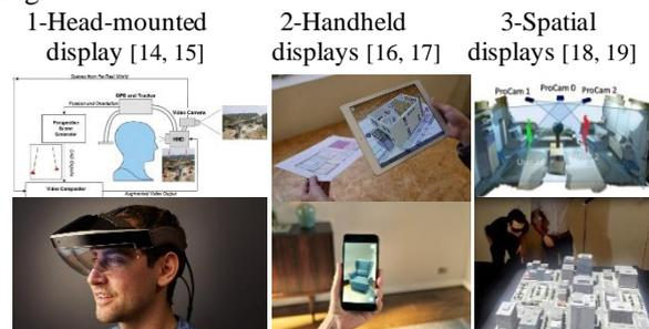
Fig.3. Different types of displays and hardware technologies used for augmented reality.
