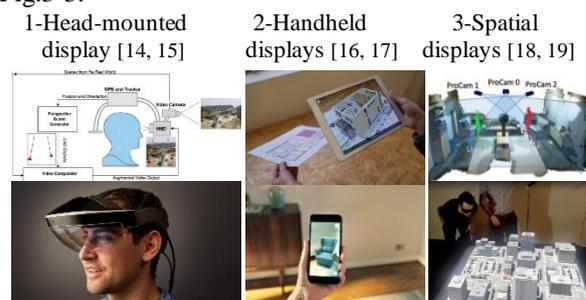
Fig.3. Different types of displays and hardware technologies used for augmented reality.
