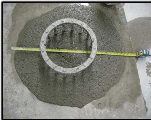
Figure (3): J-ring test
