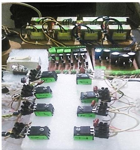
Fig. (12) Eight switches bridge converter (ESBC)
