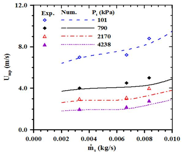
Fig. 8. Effect of total operating pressure on the minimum pressure drop velocity: comparison with experimental data of Plasynski et al. (1994).
