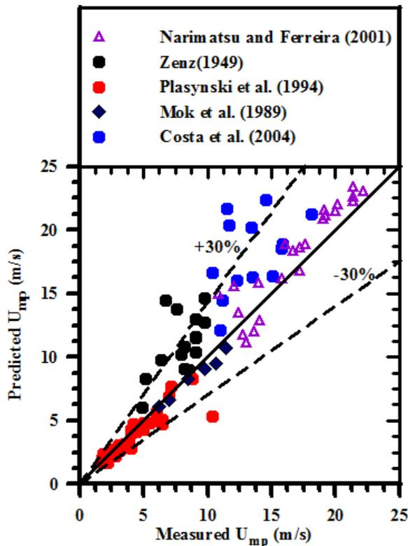
Fig. 6. Comparison between predicted and measured minimum pressure drop velocity.
