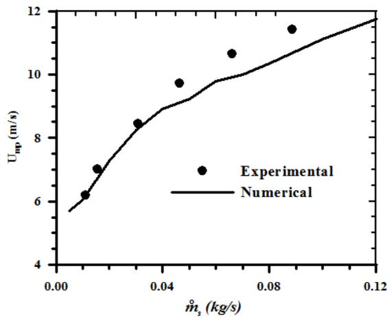
Fig. 7. Effect of solid mass flow rate on the minimum pressure drop velocity: comparison with experimental data of Mok et al. (1989).
