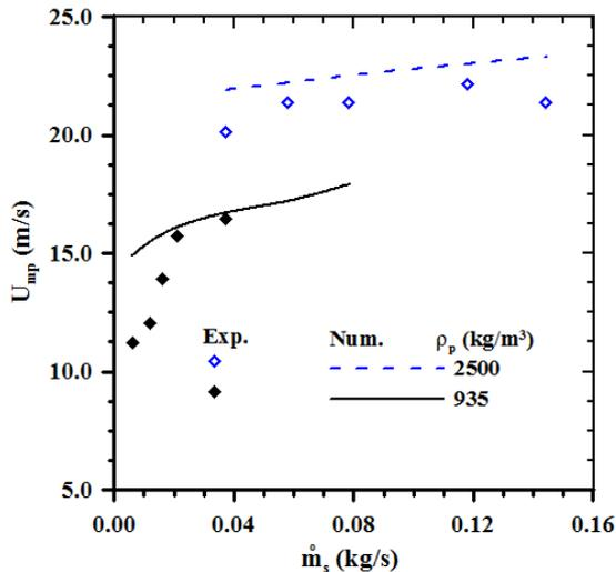
Fig. 10. Effect of particle density on the minimum pressure drop velocity: comparison with experimental data of Narimatsu and Ferreira (2001)
