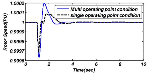
Fig. 8 Rotor speed for single and multi operating conditions
