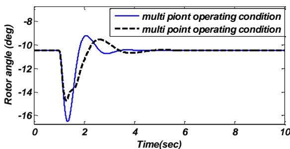
Fig. 7 Rotor angle for single and multi operating conditions
