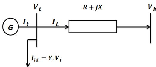
Fig. 2Single machine infinite bus
