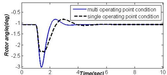
Fig. 9 Rotor angle for single and multi operating conditions
