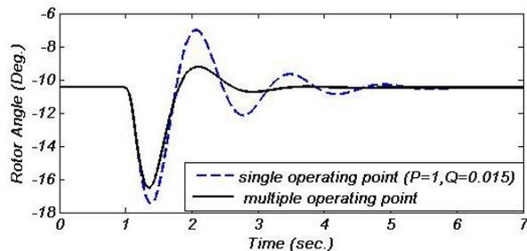
Fig. 11 A comparison between single and multiple design response for rotor angle
