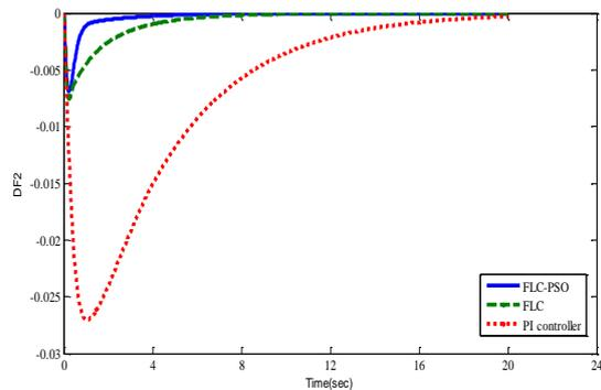
Fig. (8) Dynamic response for frequency deviation of area 2
