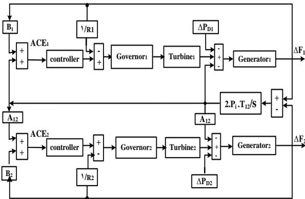
**Fig. (1)** Block diagram of two-area thermal system.
