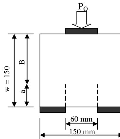
**Fig.3** Double notch cubic specimen
