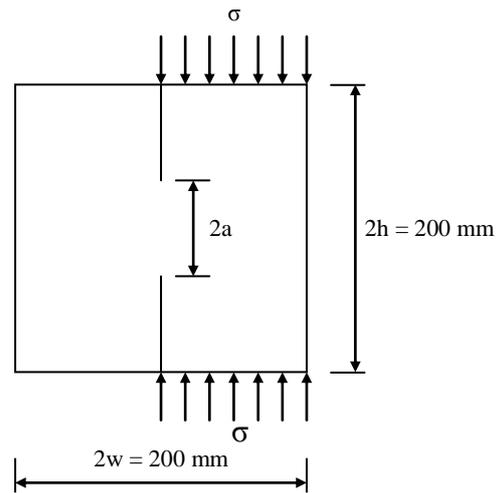
**Fig.2** Double-edge notched prism geometry.
