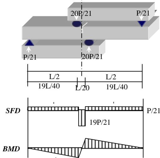
Fig.4 Four-points shear test setup
