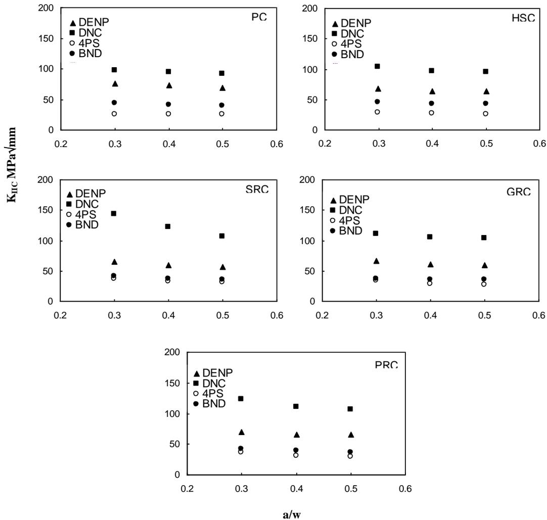
Fig.7 Notch depth to specimen width ratio (a/w) versus mode II fracture toughness  $K_{IIc}$  for different concretes.
