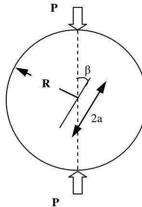
Fig.5 Cracked Brazilian disc specimen
