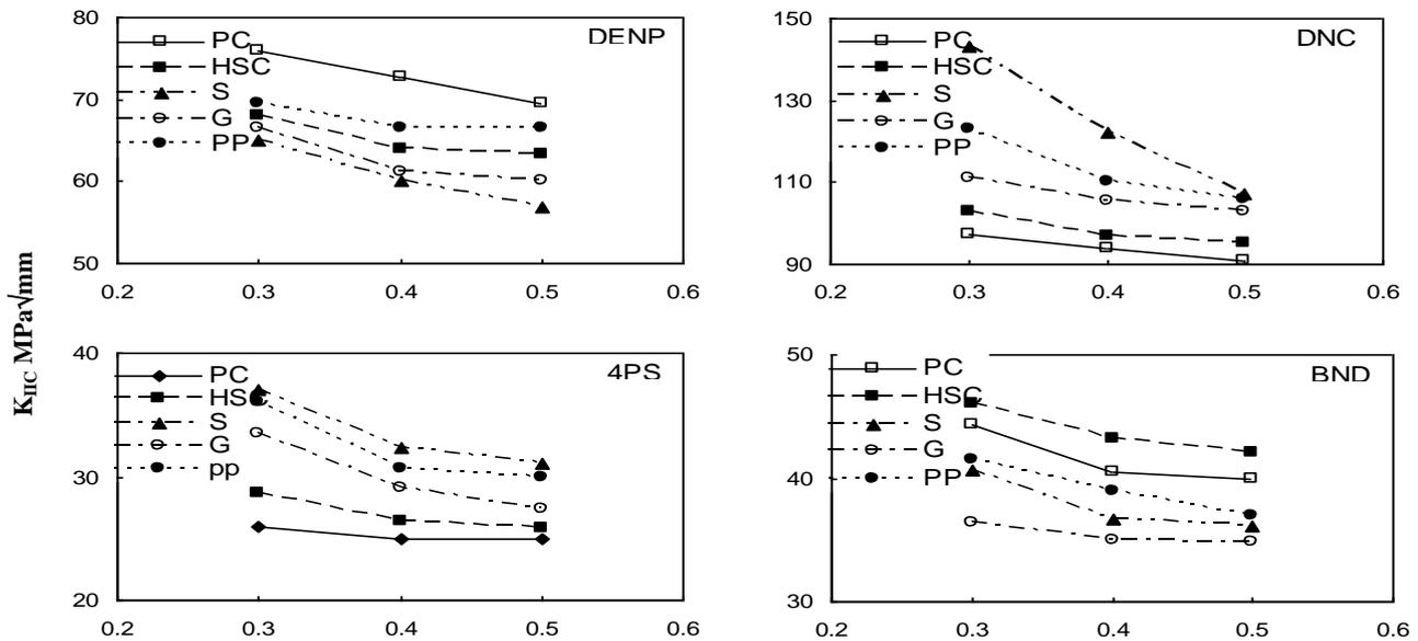
Fig.6 Notch depth to specimen width ratio ( $a/w$ ) versus mode II fracture toughness  $K_{IIc}$  for various test setups.
