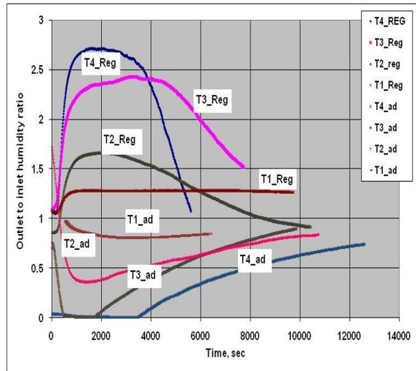
Figure (4) the variation of the outlet to inlet air humidity ratio with the adsorption or desorption time with the adsorption or desorption time for different air regeneration temperatures at air mass flow rate of 0.71 kg/min
