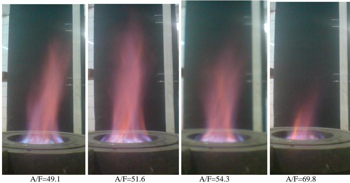
**Figure(7):** combustion run for conical stabilizer with injector have an angle of 38 degree on horizontal axis and 0 degree on vertical axis at  $v=5.06$  m/s
