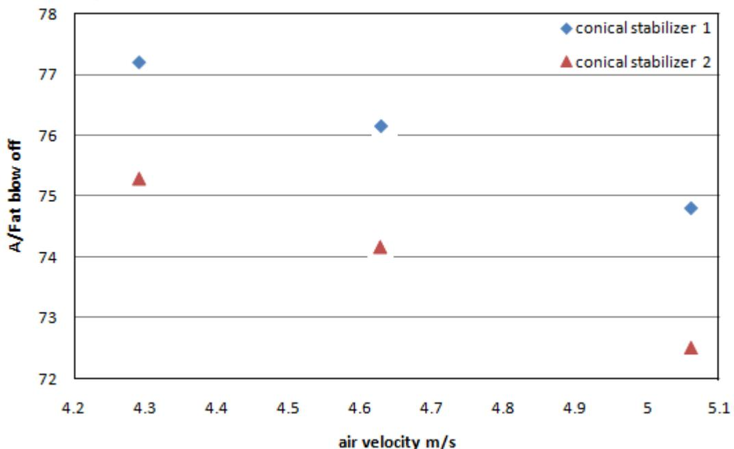
**Figure (8)** Variation of air-fuel ratio at blow off with air velocity for two design of conical stabilizer
