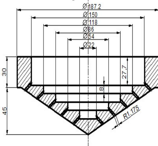
Figure (2) conical stabilizer
