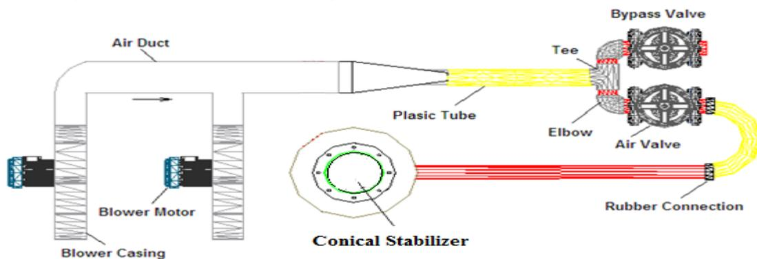
Figure (1): Plan View for Test rig System Main Parts
