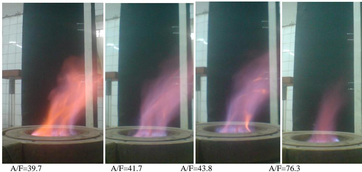
**Figure(4):** combustion run for conical stabilizer with injector have an angle of 38 degree on horizontal axis and 10 degree on vertical axis at v= 4.29 m/s
