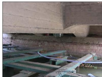
Fig. 3: Accelerometer attached to the bridge.
