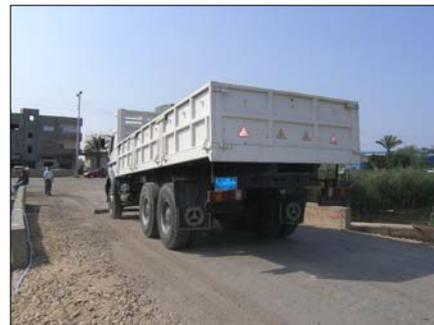
Fig. 2: Photo for the truck and the obstacle on the bridge.
