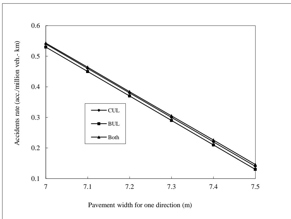
**Figure (6):** Relationship between Pavement Width and Accidents Rate for Divided Highways
