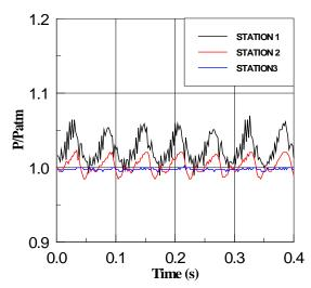
**Fig. 7** Pressure traces at initial frequency =17.75 Hz for Large cavity with absorbing materials (glass-wool) followed by small one (muffler) (LWSE1)
