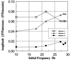
**Fig. 14** Amplitude versus Frequency (Hz) at different stations, Large cavity followed by small one with absorbing materials in both (muffler).
