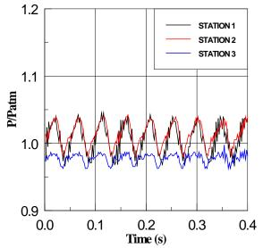
**Fig. 4** Pressure traces at initial frequency =21.57 Hz for Large cavity followed by small one (muffler) without absorbing materials (LSE2).
