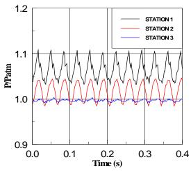
**Fig. 9** Pressure traces at initial frequency =29.13 Hz for Large cavity with absorbing materials (glass-wool) followed by small one (muffler) (LWSE3)
