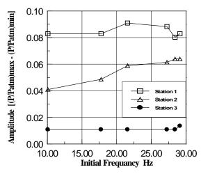
**Fig. 13** Amplitude versus Frequency (Hz) at different stations, Large cavity with absorbing materials followed by small one (muffler)
