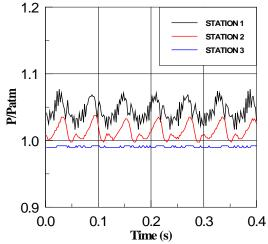
**Fig. 10** Pressure traces at initial frequency =17.75 Hz for Large cavity followed by small one with absorbing materials in both (muffler) (LWSW1)
