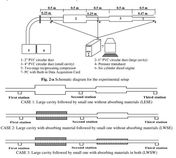
Fig. 2-b Schematic diagram for three test cases
