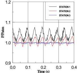
**Fig. 8** Pressure traces at initial frequency =21.57 Hz for Large cavity with absorbing materials (glass-wool) followed by small one (muffler) (LWSE2)
