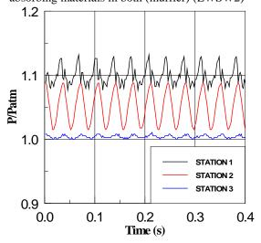
**Fig. 12** Pressure traces at initial frequency =29.13 Hz for Large cavity followed by small one with absorbing materials in both (muffler) (LWSW3)
