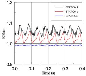
**Fig. 11** Pressure traces at initial frequency =21.57 Hz for Large cavity followed by small one with absorbing materials in both (muffler) (LWSW2)
