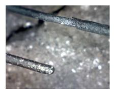
**Fig. 7** Oxidation of SF at 600 <sup>o</sup>C
