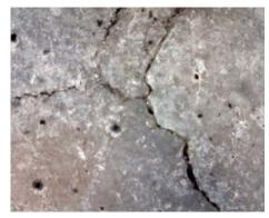
Fig. 8 Severe cracking at 750 °C
