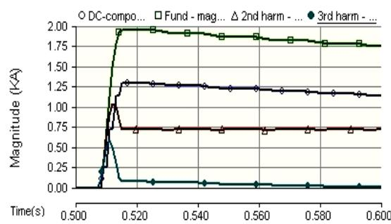
**Fig. 13** FFT magnitudes for current in Ph (C).
