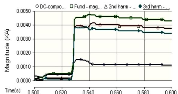
**Fig. 21** FFT magnitudes for current in Ph (C).
