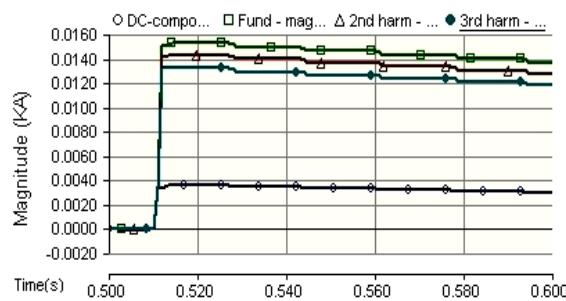
**Fig. 9** FFT magnitudes for current in Ph (C).
