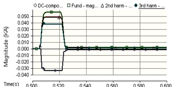
**Fig. 7** FFT magnitudes for current in Ph (A).
