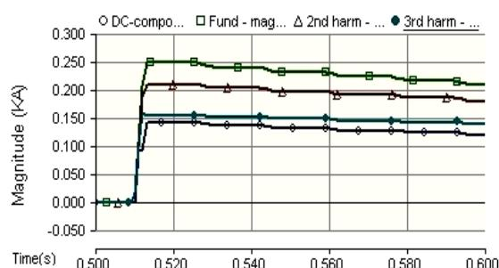
**Fig. 5** FFT magnitudes for current in Ph (C).
