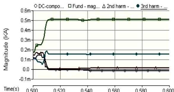
**Fig. 19** FFT magnitudes for current in Ph (A).
