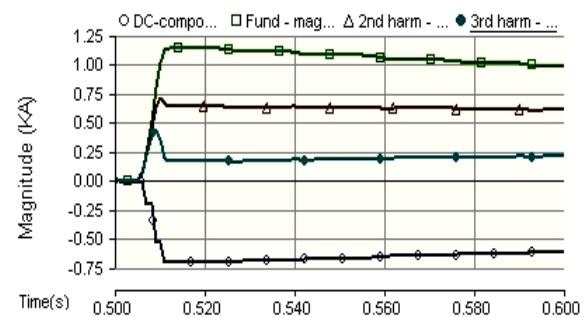
**Fig. 11** FFT magnitudes for current in Ph (A).
