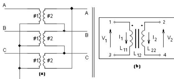
**Fig. 1** PSCAD/EMTDC model (a) 3-phase, 2-winding transformer (b) classical modeling approach
