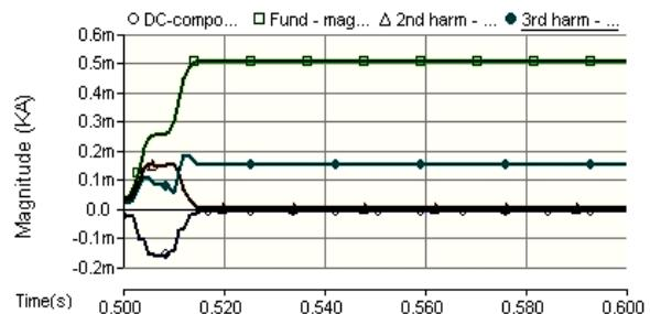
**Fig. 17** FFT magnitudes for current in Ph (C).
