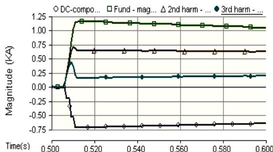
**Fig. 3** FFT magnitudes for current in Ph (A).
