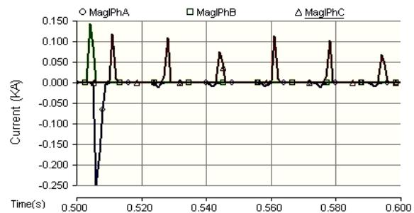
**Fig. 6** Elimination of inrush current using pre-insertion resistor
