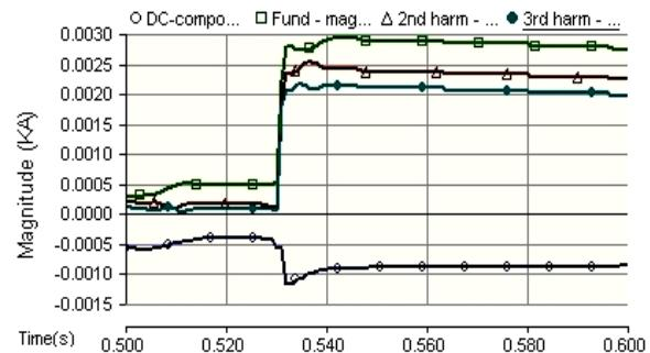
**Fig. 20** FFT magnitudes for current in Ph (B).
