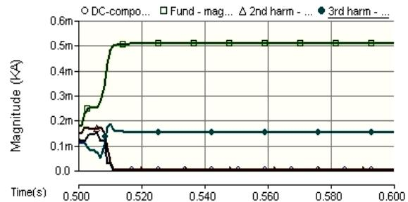
**Fig. 16** FFT magnitudes for current in Ph (B).
