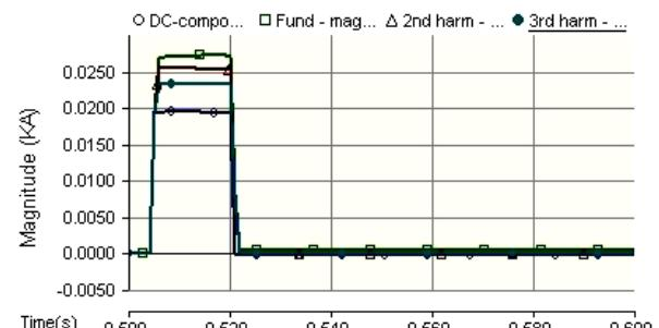
**Fig. 8** FFT magnitudes for current in Ph (B).
