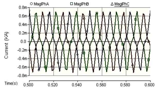
**Fig. 14** Reduction of Inrush with no residual flux.
