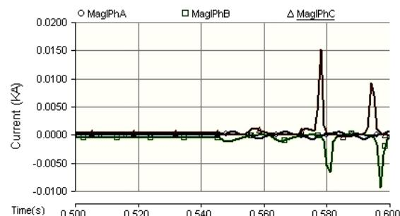
**Fig. 22** Reduction of Inrush with residual flux by delay closing strategy.
