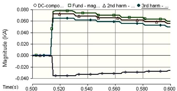
**Fig. 12** FFT magnitudes for current in Ph (B).
