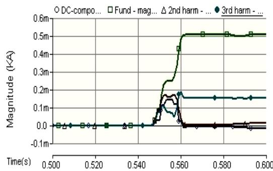
**Fig. 23** FFT magnitudes for current in Ph (A).
