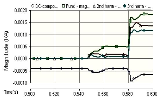
**Fig. 24** FFT magnitudes for current in Ph (B).
