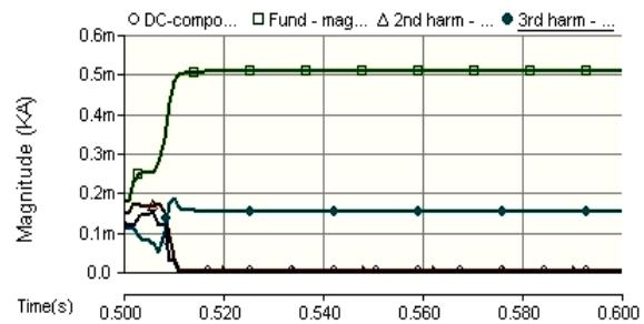
**Fig. 15** FFT magnitudes for current in Ph (A).
