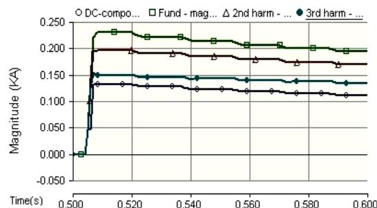
**Fig. 4** FFT magnitudes for current in Ph (B).
