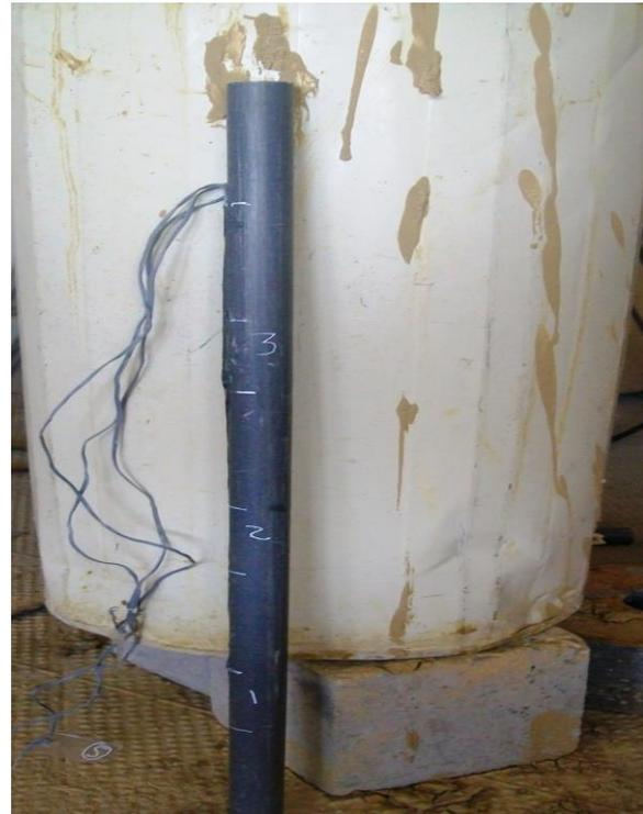
Photo (1): The model pile with strain gauges.
