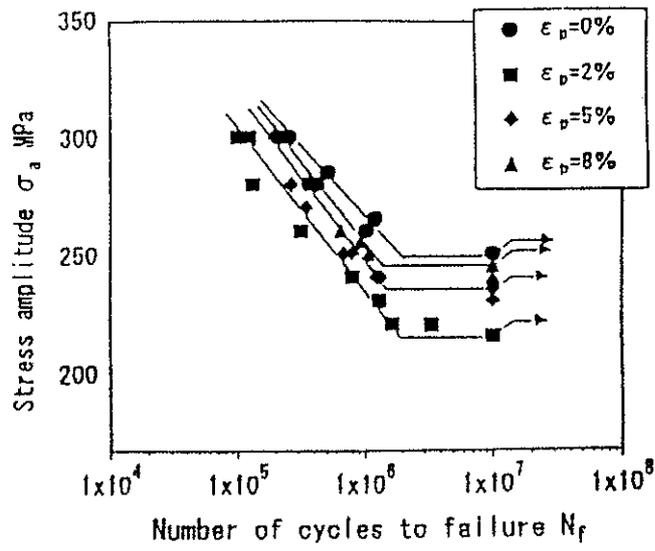
Fig. 5 S-N curves of material B(0.46%C).
