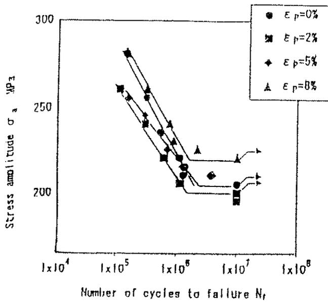
Fig. 4 S-N curves of material A (0.15% C).
