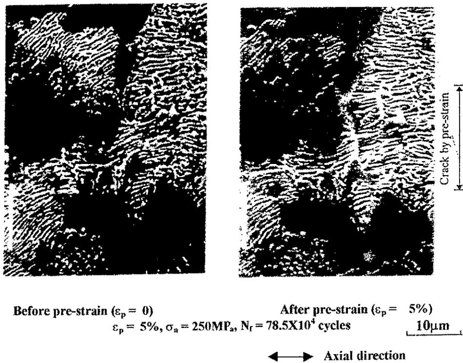
Fig. 10 Successive observation of fatigue crack initiation of pre-strained specimen using SEM (material B:0.46%C).
