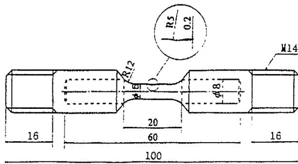
Fig. 1 Shape and dimensions of specimen. mm.
