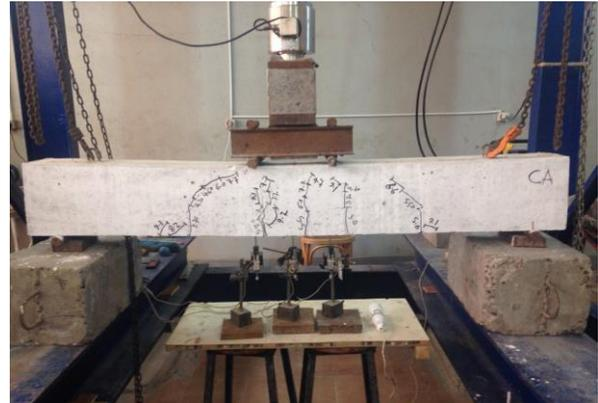
Fig.7: The mode of failure observed for beam 3.
