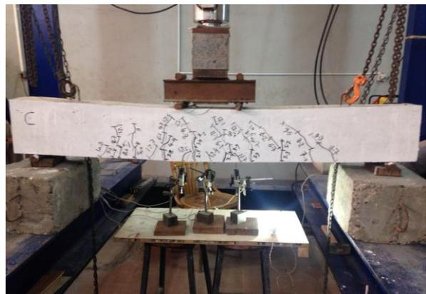
Fig.5: The mode of failure observed for beam 1
