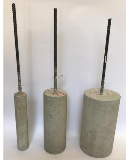
Fig.1: Corrosion test specimens.
