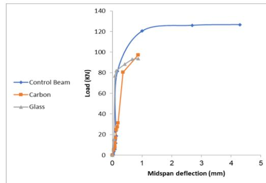
Fig.8: Load v/s deflection in beam specimens.
