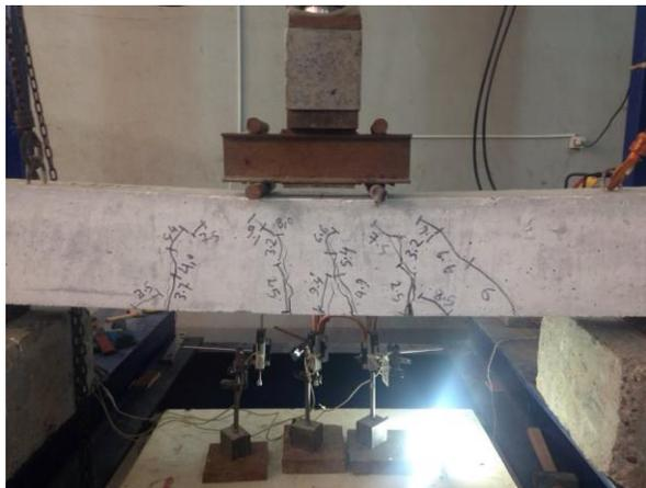
Fig.6: The mode of failure observed for beam 2.
