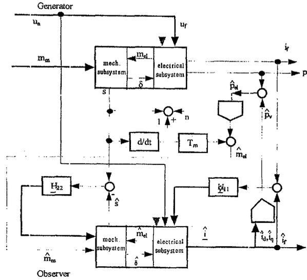
Figure (2) The synchronous generator model and its nonlinear state observer
