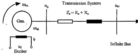
Figure (1) Synchronous Generator Model Connected To Infinite Bus
