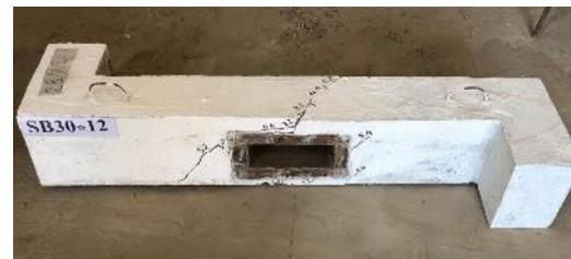
(b) Crack pattern for SB30x12
