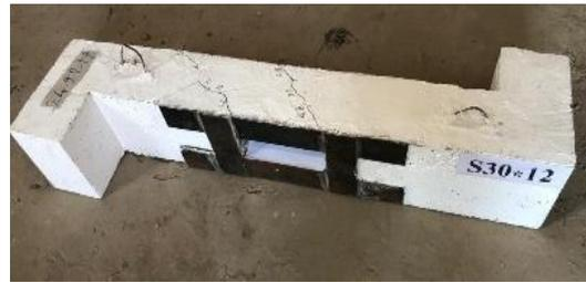
(b) Crack pattern for S30x12
