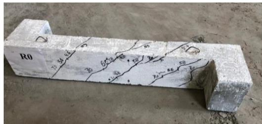
(a) Crack pattern for beam R0
