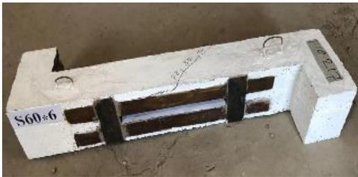
(c) Crack pattern for S60x6
