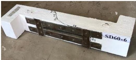
(c) Crack pattern for SD60x6
