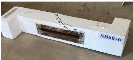
(c) Crack pattern for SB60x6
