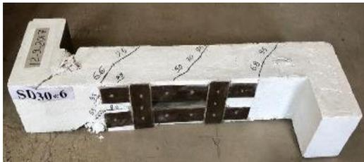
(a) Crack pattern for SD30x6
