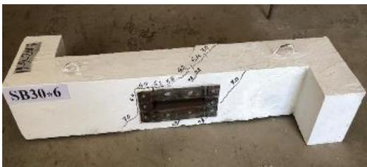
(a) Crack pattern for SB30x6
