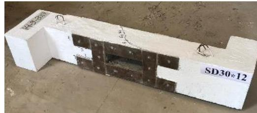
(b) Crack pattern for SD30x12
